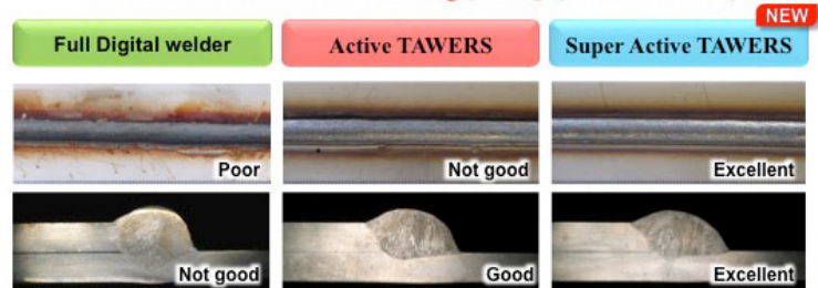
welding current: 250A, welding speed: 100 cm/min, shielding gas: Ar98% + CO 2 , base metal: stainless steel 304, plate thickness: 2,0 mm, joint: lap, wire: 308LSI (Ø1,2)
