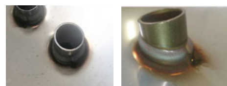
welded with CMT process
