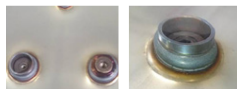
welded with Super Active Wire Process
