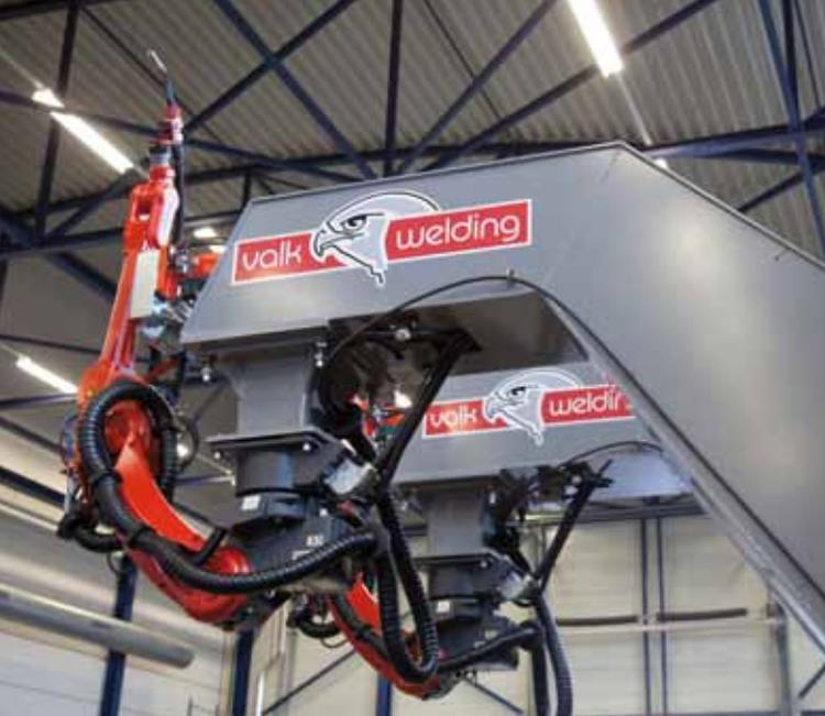
Valk Welding supplied a robot system for the production of single piece composite beams for Danish steel construction company
