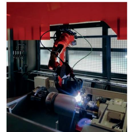
components are controlled by 1 CPU) we decided to continue with Valk Welding," says Michael Bourhenne. Tailored to the requirements of Eagle Burgmann, a concept was developed based on a turntable solution with 2 C-manipulators and freely programmable turning and tilting functions. The TL-1800 WG3 welding robot has been set up at a working angle to make clamping the large pressure vessels and assemblies as ergonomic as possible.
