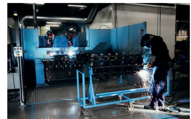
In the meantime, while the operator is waiting for the welding robot, the operator performs a manual welding operation.
