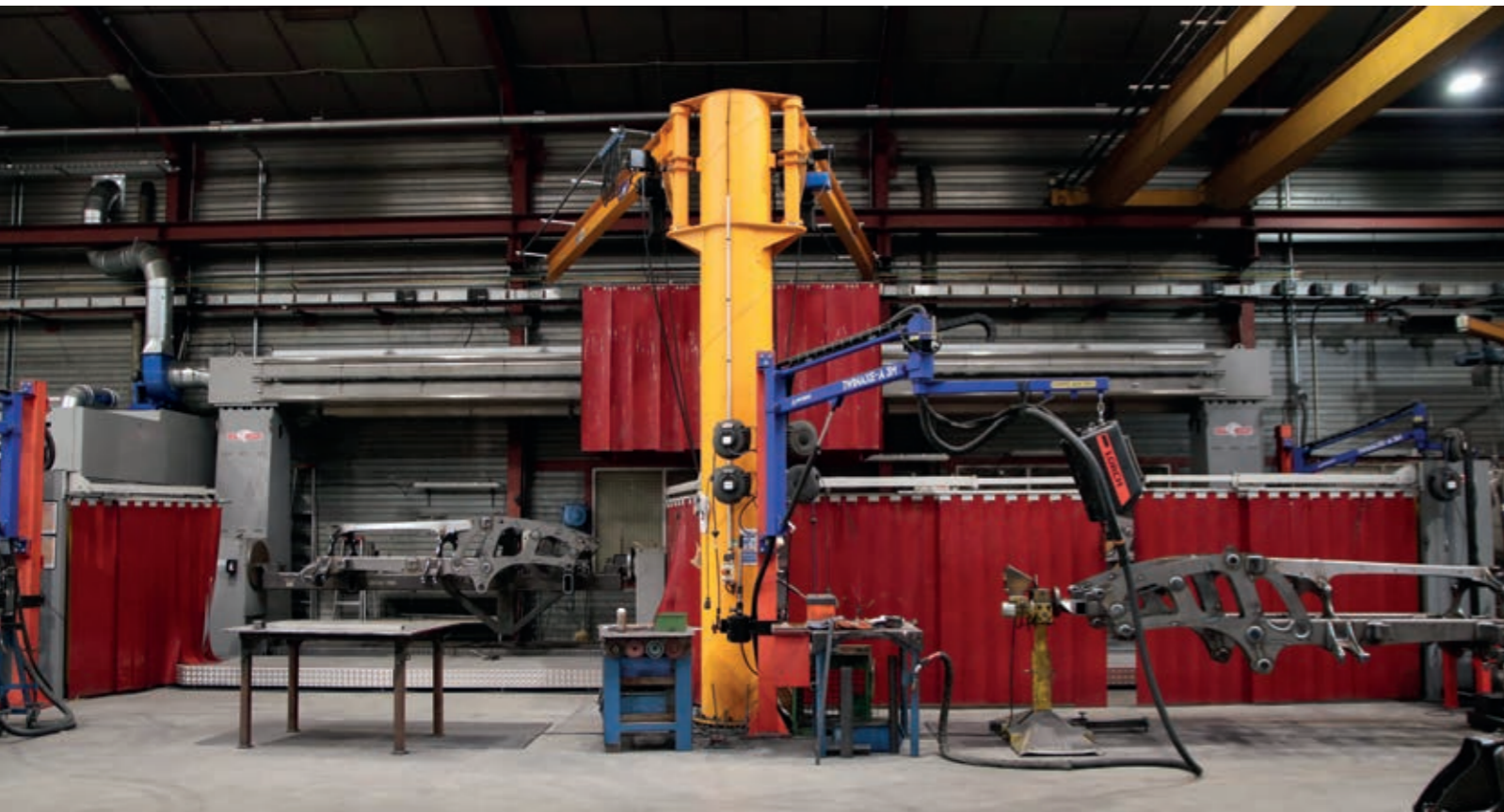
The first cell developed by Valk Welding for Comebo Industries is based on a suspended robot on a gantry, for dimensions up to 5 metres, instead of 3.2 metres with the previous machine.
