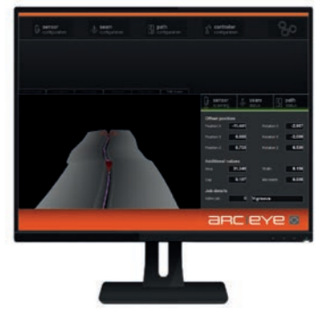
3D Seam-Tracking: during the weld seam tracking, the robot is guided through a 3D scanned landscape.
