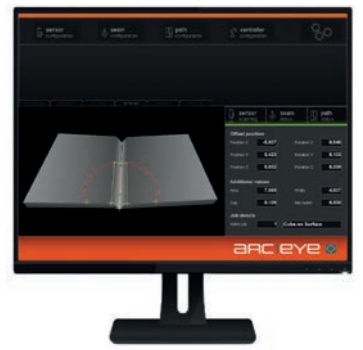
3D Seam-Finding (start of a weld seam): in the above image, the starting point, direction and dimensions of the V-groove are searched and found in one query.
