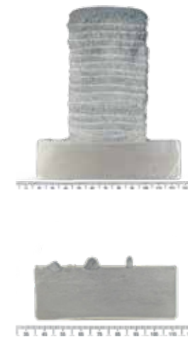
Figure 1. Scale up process from single beads to 3D printed block
