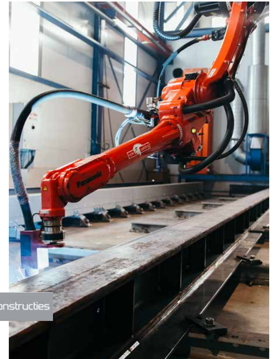
The robot now welds 15 m long SFB composite corner beams in 3 hours
