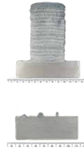
Figure 1. Scale up process from single beads to 3D printed block
