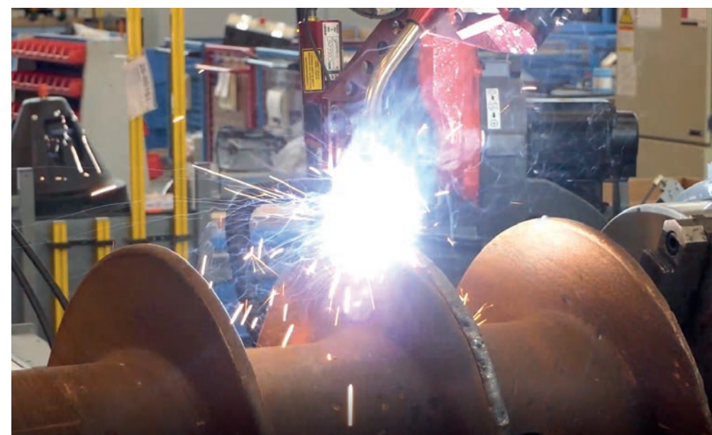
Wear application of several layers, up to 30 mm
