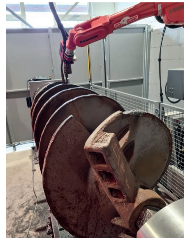
Arc-Eye takes over the path guidance
