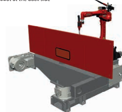
FRAME-IT+H with turning table and robot at the back side
