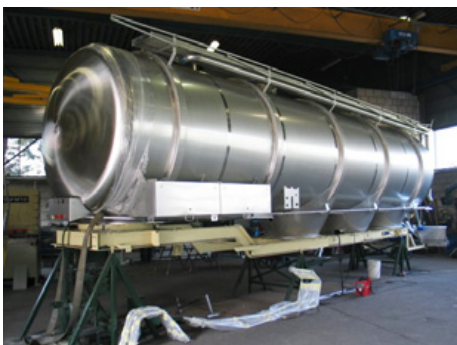
The RVS liquid tanks which are welded through automation by Hazeleger with the longitudinal and round-seam welding machine from ADK Techniek.
