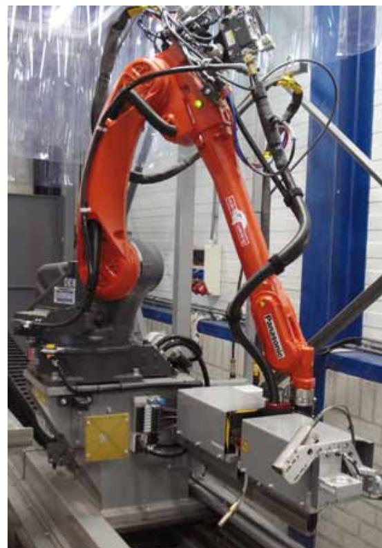
robotisation. The manufacturer previously invested in a welding robot system in 1996 and is among the first users of the offline programming package Desktop Programming & Simulation (DTPS) in de Benelux region. Marel Stork Poultry Processing also uses Panasonic robots for other processes such as the glass pearlizing of products.
