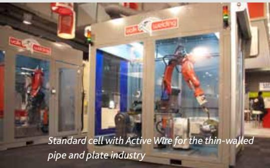
Standard cell with Active Wire for the thin-walled pipe and plate industry
