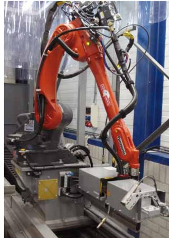
robotisation. The manufacturer previously invested in a welding robot system in 1996 and is among the first users of the offline programming package Desktop Programming & Simulation (DTPS) in de Benelux region. Marel Stork Poultry Processing also uses Panasonic robots for other processes such as the glass pearling of products.
