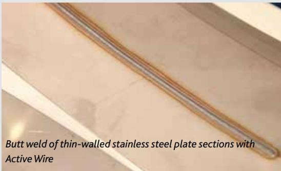
Butt weld of thin-walled stainless steel plate sections with Active Wire
