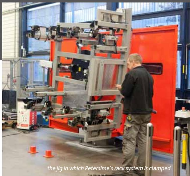
*the jig in which Petersime's rack system is clamped*
