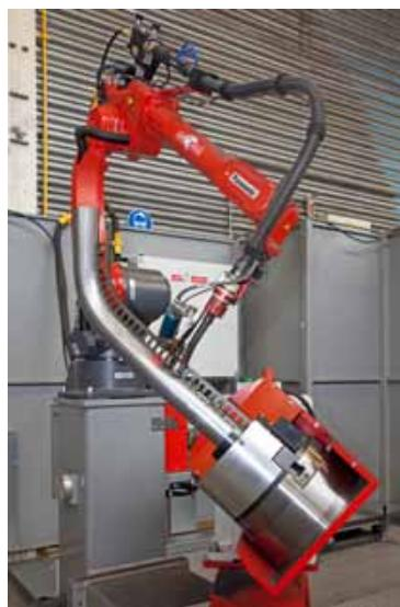
for the welding robot from CAD and ERP databases. This means robot automation can be used for single item production without needing a programmer and client-specific products can be produced in a serialized manner in accordance with the principle of Mass Customization.
