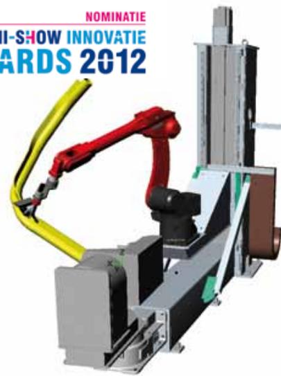
for the welding robot from CAD and ERP databases. This means robot automation can be used for single item production without needing a programmer and client-specific products can be produced in a serialized manner in accordance with the principle of Mass Customization.
