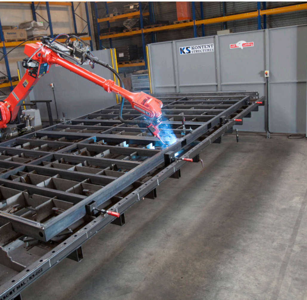
The Panasonic HH-020L welding robot has an exceptional reach of 3281 mm
