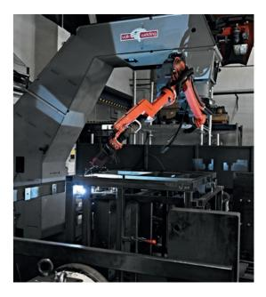
two TRACK-FRAME-E-type robotic systems for welding other flat subassemblies, and one robotic system with a hanging robot for welding large subassemblies and complete 3D assemblies.
