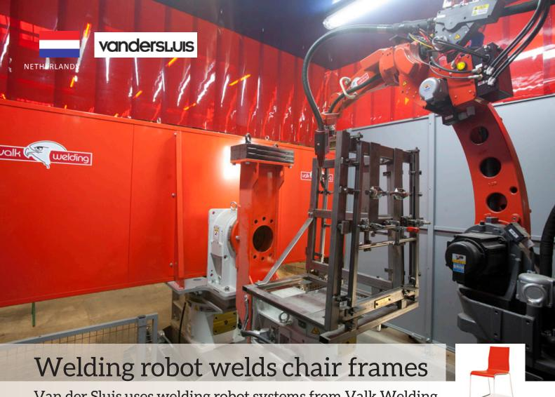
Van der Sluis uses welding robot systems from Valk Welding
