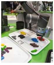
the TM-cobot is always able to determine the right exact position. And the gripper will always pick up a product in the centre or as programmed. Therefore, these products do not need to be placed in pre-programmed positions. TM-cobots first scan the location and then determine their exact position. That provides an enormous programming convenience, and saves a significant amount of programming time."
