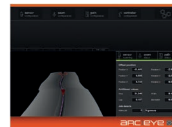
3D Seam-Tracking: During weld seam tracking, the robot is guided through a 3D scanned landscape.
