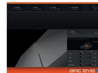
3D Seam-Analysis: The weld seam is analysed and checked in a 3D view.
