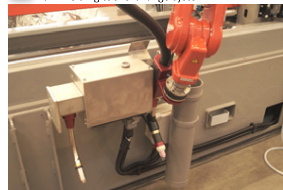
The welding robot switches automatically between the MIG and TIG torch
