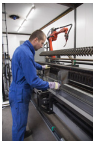
LEDs on the jig show where the operator has to place the holders.
