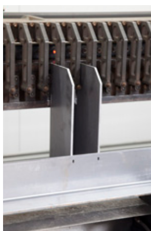
LEDs on the jig show where the operator has to place the holders.
