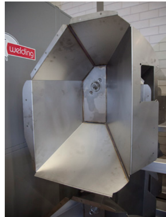
A stainless steel product welded on the outside and completely welded through to the inside
