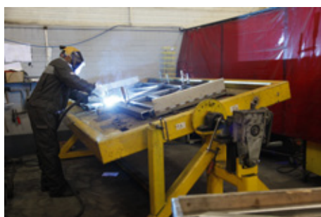
Cross sections were welded manually until recently
