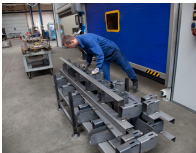
The holders are placed on the girders without pre-attachment.
