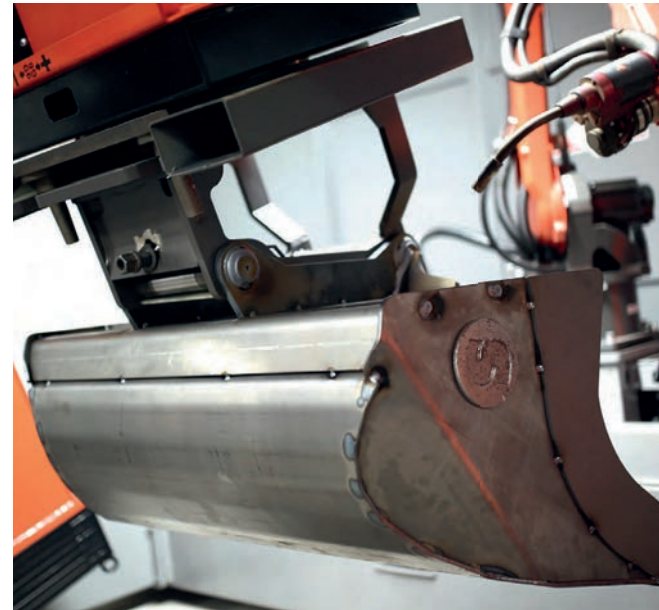
Extensive development work has been done on the fixture systems to achieve the most automated welding process possible.
