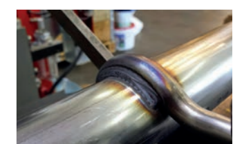
HD-MAG welding process
