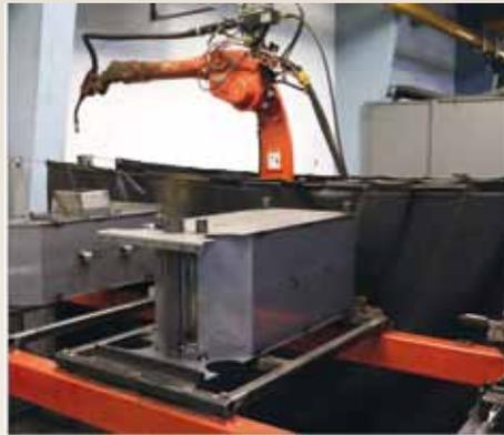
The welding robots form a vital component in the production of the 60,000 wood pellet stoves that Rustek delivers each year.
